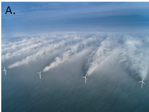
Figure 3: A. Front-on view of the Horns Rev wind farm (Vattenfall; Photo: Christian Steiness). B. Numerical simulation [4]
