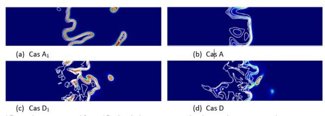
2D sections extracted from 3D simulations representing heat release rate and temperature iso-surfaces
