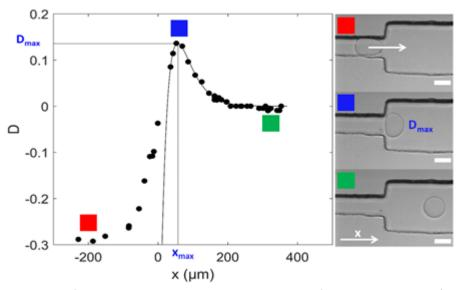
Deformation of a droplet passing through a microfluidic restriction (at x=0). On the images to the right, the white line represents 100  $\mu$ m.
