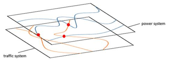
Principle of overlaying the traffic system diagram and the electrical network diagram used in the optimization model
